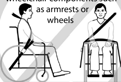
Figure 3a - Improper positioning of pelvic-belt restraints over wheelchair supports.
