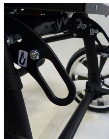
Attachment points, rear according to ISO 7176-19
